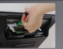
CPU module can be accessed without removing any peripherals or wires for quick serviceability.
